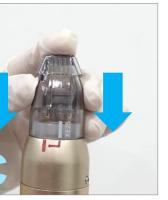
Align the line of the tip with the L-shaped line of the handpiece and connect while pressing.
